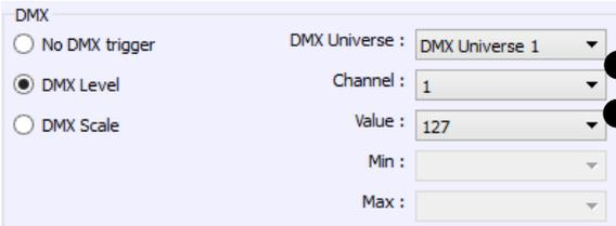
The screenshot shows the DMX Level configuration interface. It includes three radio buttons: 'No DMX trigger', 'DMX Level' (which is selected), and 'DMX Scale'. To the right, there are four dropdown menus: 'DMX Universe' (set to 'DMX Universe 1'), 'Channel' (set to '1'), 'Value' (set to '127'), and 'Min' (empty). A 'Max' dropdown is also present but empty.
