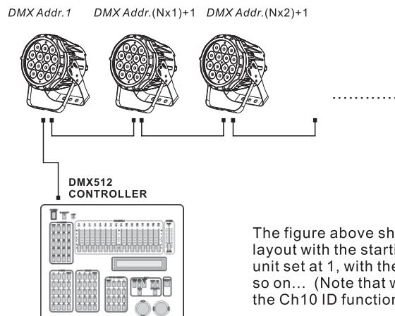
The figure above shows a simple DMX512 layout with the starting address of the first unit set at 1, with the second set at  $(Nx1)+1$  and so on... (Note that when used in this way, the Ch10 ID function must be inactive (CH10=0))
