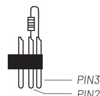
When using standard DMX512 control signal, the last device's output interface must be connected to a DMX plug. This plug is putting a 120 ohm resistance between "canon" plug's 2 pin and 3 pin. Showing as below pic. Sticking this plug into the last device's signal output interface, it will avoid the interference during the process of signal transmission.
