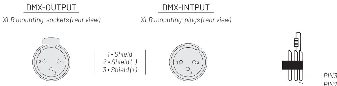
When using standard DMX512 control signal, the last device's output interface must be connected to a DMX plug. This plug is putting a 120 ohm resistance between "canon" plug's 2 pin and 3 pin. Showing as below pic. Sticking this plug into the last device's signal output interface, it will avoid the interference during the process of signal
